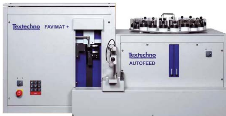
Fig. 4: FAVIMAT+ AUTOFEED (without TESTCONTROL computer system)
