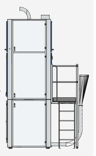
Electronic camera-based foreign matter separator installed in the cotton cleaning line
