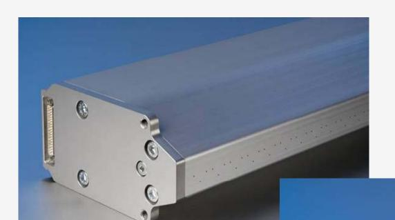
Contaminant ejection with 144 compressed air nozzles, individually controllable via 48 solenoid valves. Integrated pressure tank
