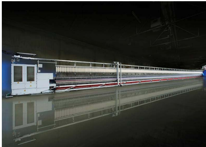
Figure 32: Zinser 351 with 1,680 spindles
