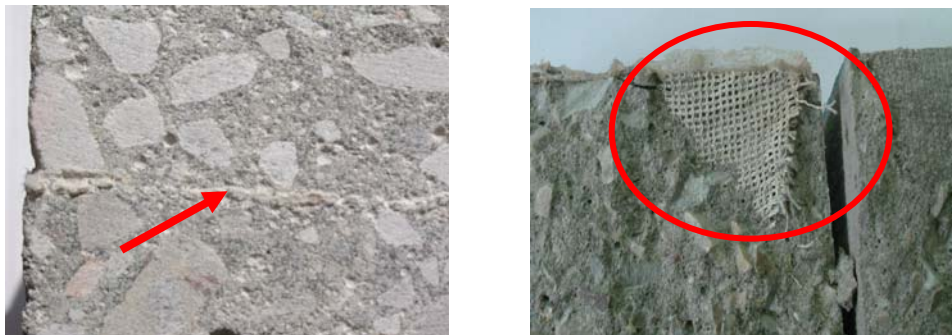
Figure 6: Building composite with cotton/PES component
