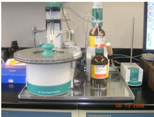
Figure 4: Example of a chemical moisture method, MetroOhm
