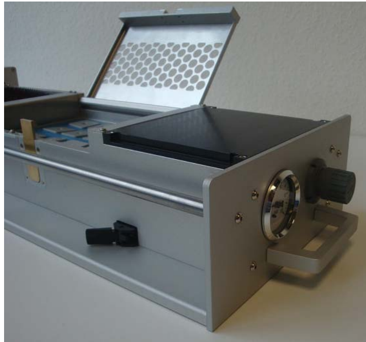
Fig. 4: Front view with regulator and lever for upwards movement
