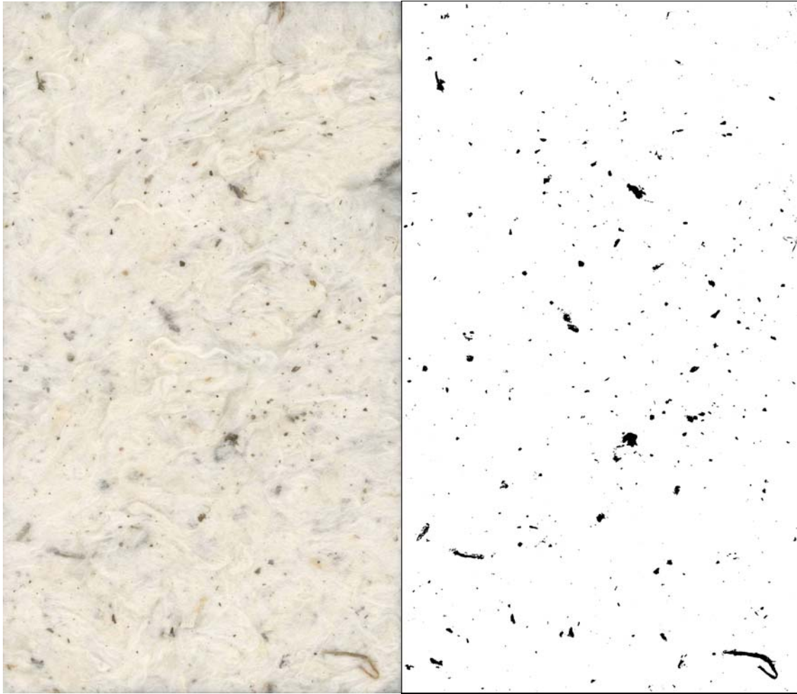
Figure 2: Cotton sample image with its thresholded binary image.
