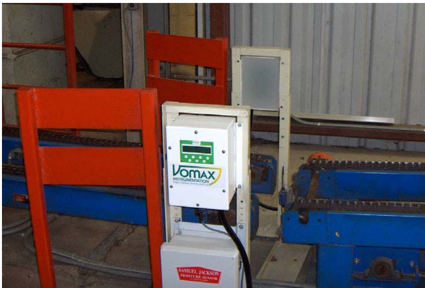
Figure 5: Microwave bale moisture measurement at the gin, Vomax 851-B
