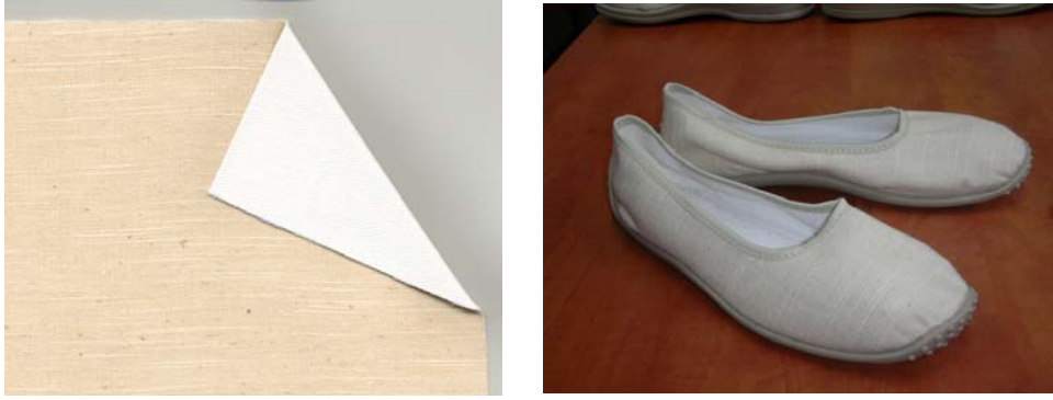
Figure 7: Cotton fabric as an upper layer of the multilayer textile materials for footwear
