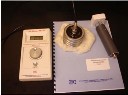
Figure 2: Example of a dielectric/conductance moisture method, Strandberg M-400 (Yarn and Surface Probes).
