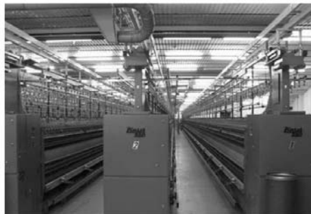
Old ring spinning installation from Zinser
