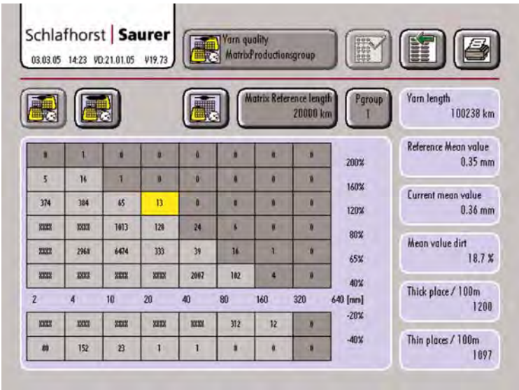
Fig. 6: Grading matrix of a weaving yarn for thick places, thin places and clusters
