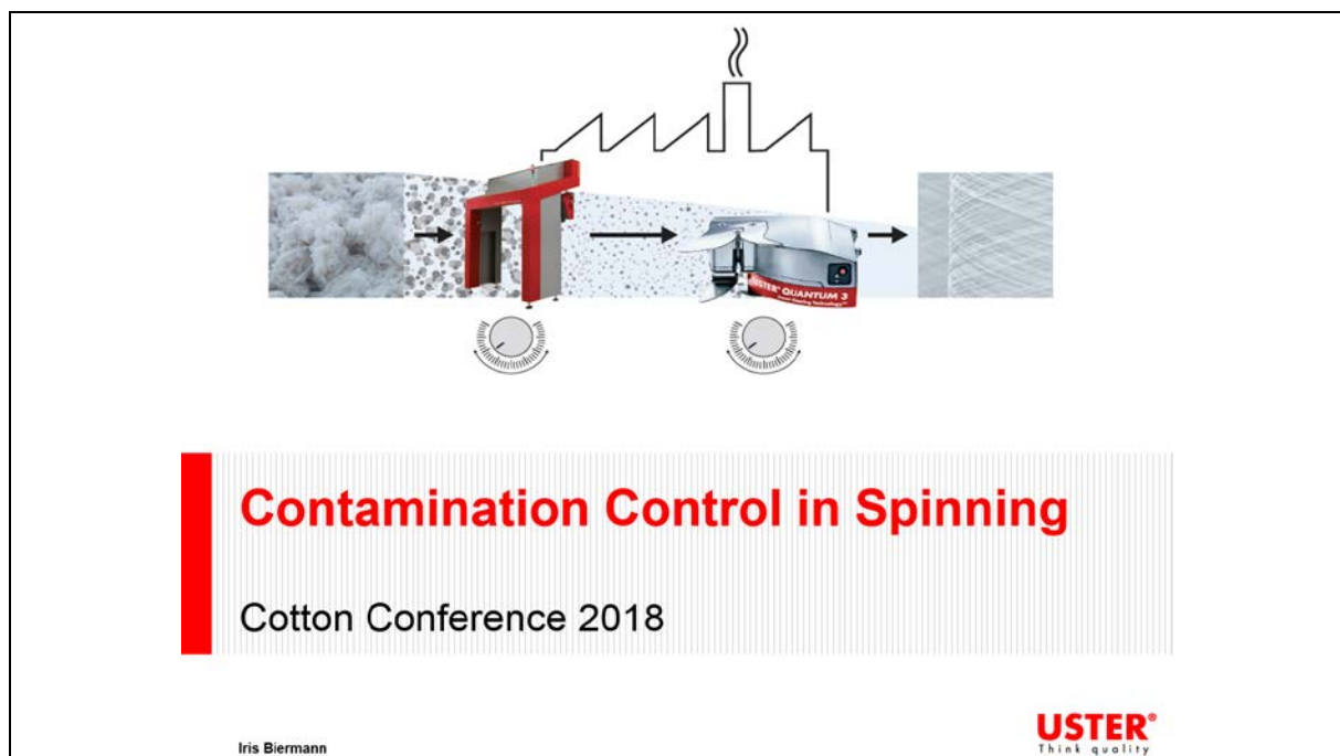
Fig. 1 Initial control with USTER® JOSSI VISION SHIELD and final control at winding with USTER® QUANTUM 3
