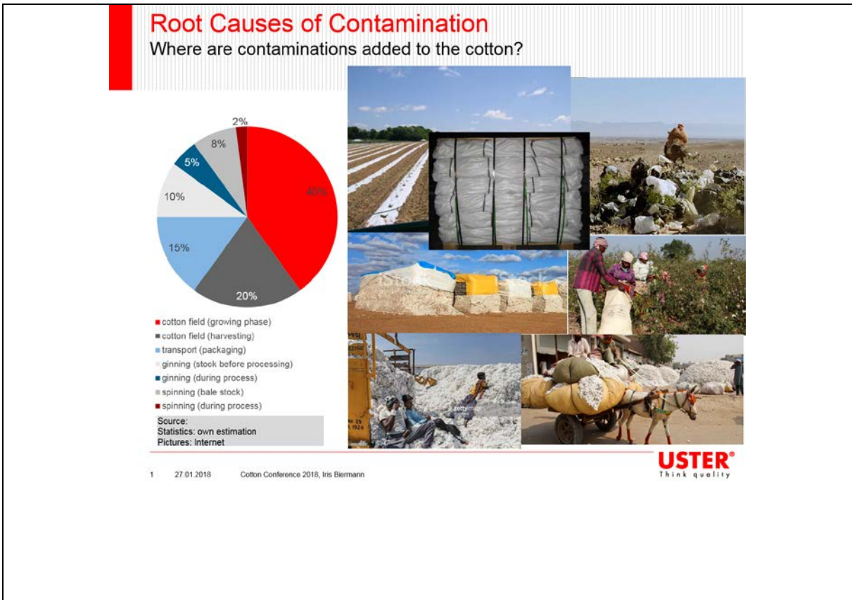
Fig. 2 Root causes of contamination
