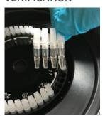
The verification is done using a qPCR test. The technology works as a key-lock system that requires the knowledge of the DNA code to detect it. The results are then uploaded into an existing ERP system, blockchain or customized digital interface. Information about the origin of the product can also be shared with the end consumer using a QR code that leads to a dedicated website.
