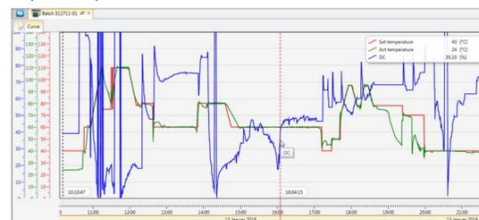
Blue curve shows turbidity measurement using DyeControl
