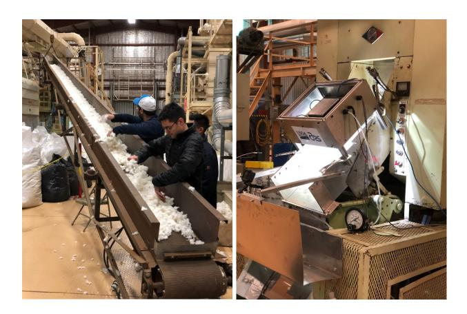
**Figure 3.** Testing of the plastic in cotton contamination detection-ejection system prototype laboratory apparatus.
