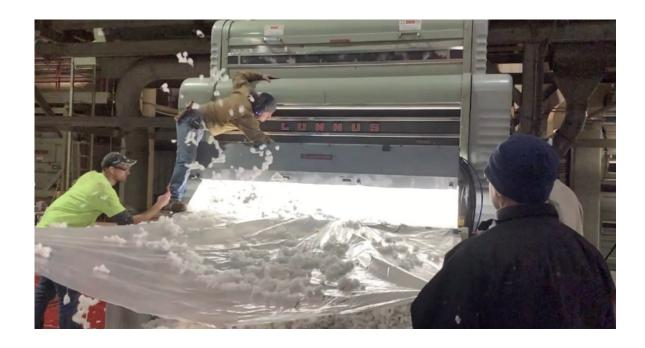
**Figure 8.** Commercial version of the USDA-ARS plastic-contamination-ejection system; as deployed into commercial cotton gin for testing and evaluation.
