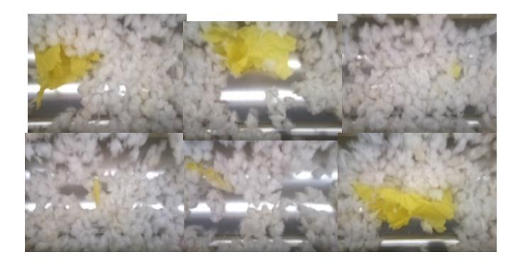
**Figure 7.** Plastic contamination detected by the prototype under deployment in a commercial cotton gin.
