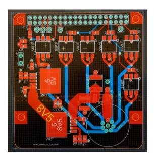
**Figure 1.** Circuit board designed to provide optically isolated high-current drive interface for the ARM micro-processor to drive the pneumatic solenoids as well as power regulation and filtering from noisy industrial environment.
