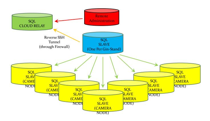
**Figure 4.** Distributive control scheme that allows for setup and configuration of multiple camera nodes from a single remote monitor.
